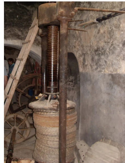
Working screw press, by a.froese – alte Olivenpresse, CC BY-SA 2.0.
